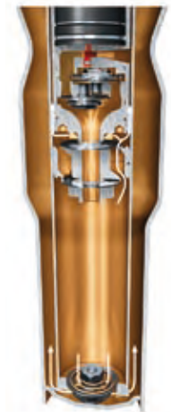
Compression in 'Sport' mode – working piston only, sporty-hard tuning
