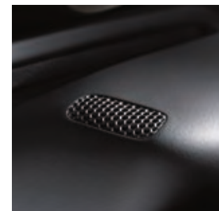
Microphone for AudioPilot® on the steering column
